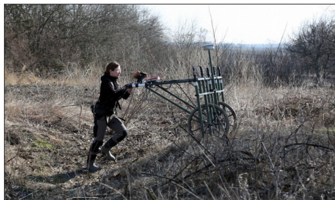
Fig. 5. Prospecting with the 14-channel system in the valley of the River Boyne in Ireland (J. Kalmbach)
