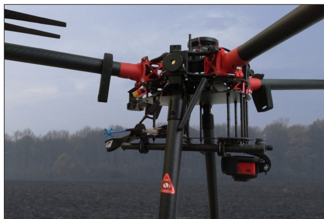
Fig. 3. Pre-flight preparation of a drone at Öcsöd-Kováshalom in the Tisza region. The fully pre-programmable drone was equipped with a multispectral sensor (H. Höhler-Brockmann)
