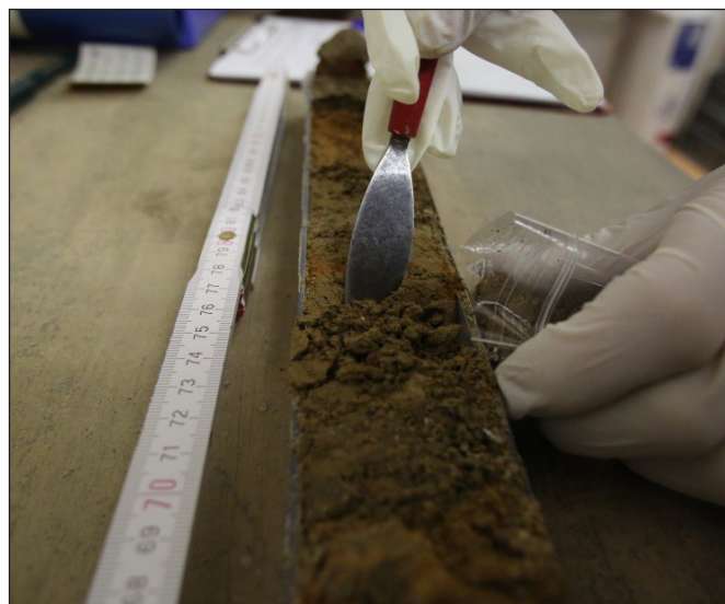
Fig. 6. Layer sequence of a soil core. The halved core is ready for documentation and for the sampling of certain layers (J. Kalmbach)
