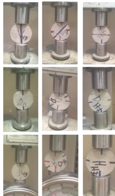
Figure 4. Procedure of OITS test on sandstone disk sample
