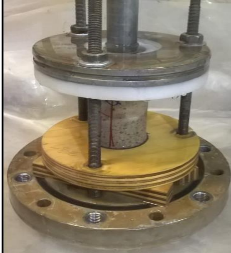
Figure 4-3. RLM sample during drilling using a diamond coring drill bit
