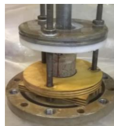
Figure 3. Sample holder while coring a 47.6 mm RLM sample using 25.4 mm impregnated diamond coring bit
