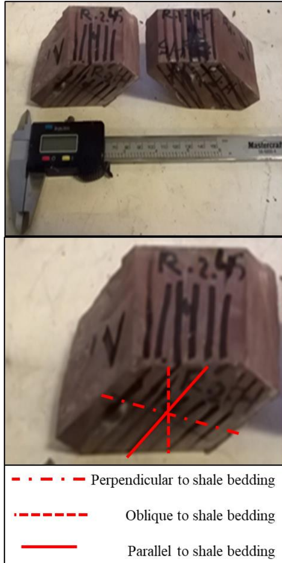
Figure 2-4. Cube shape technique for VP and VS measurement from the same hexagon shale samples
