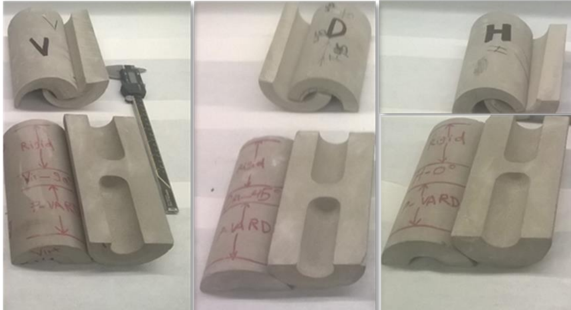
Figure 9-12. Strength samples' source (top) drilled samples using compliant and non-compliant drilling (bottom)
