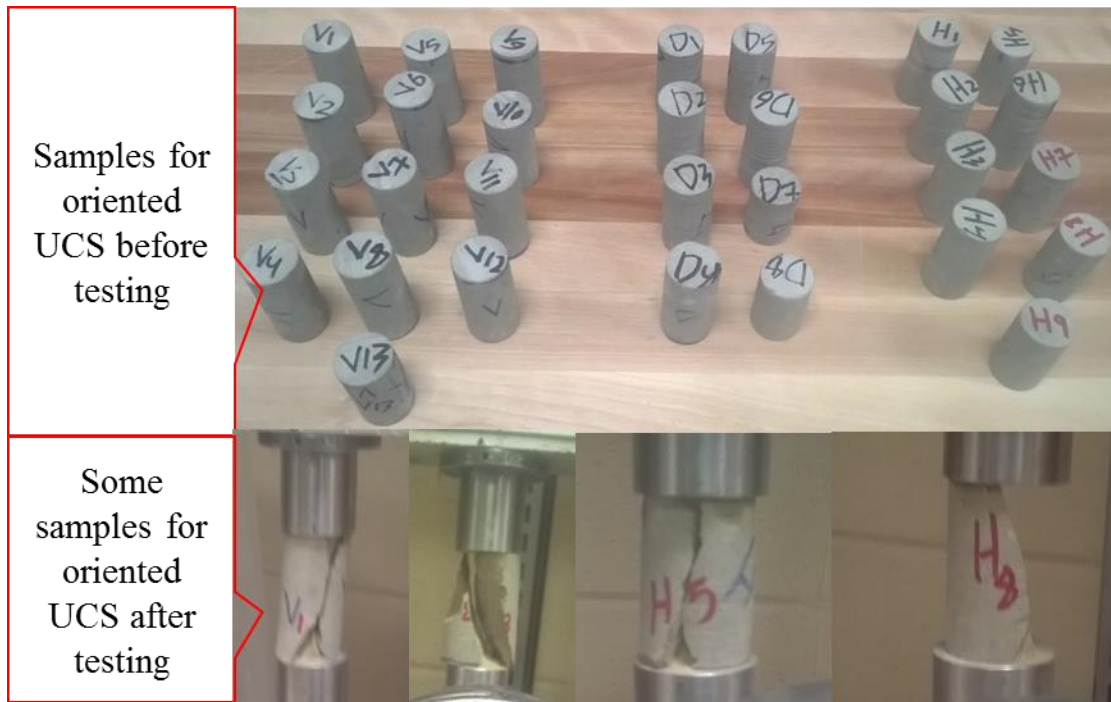
Figure 9-6. Samples before (top) and after (bottom) performing OUCS test showing a consistent shear fracture pattern
