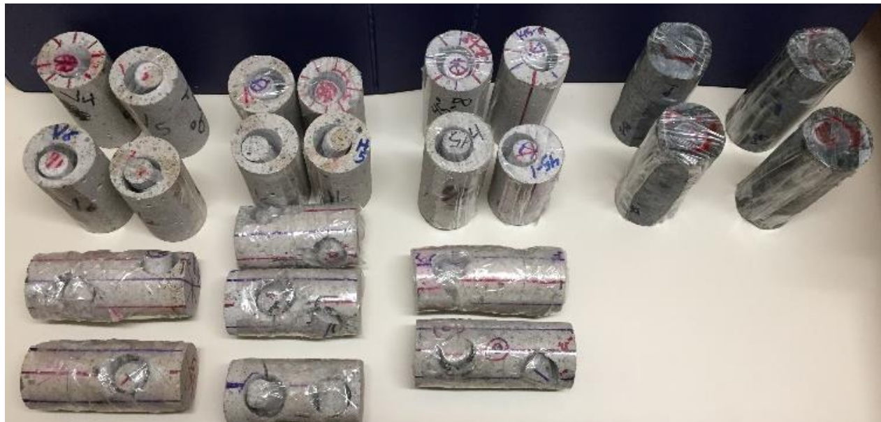
Figure 4. 47.6 mm RLM and granite samples after coring by 25.4 mm diamond impregnated coring bit in different orientations
