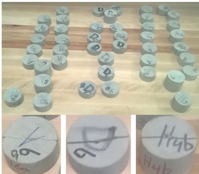
Figure 9-7. Samples before (top) and after (bottom) performing the OPLS test and showing consistent valid fracturing modes
