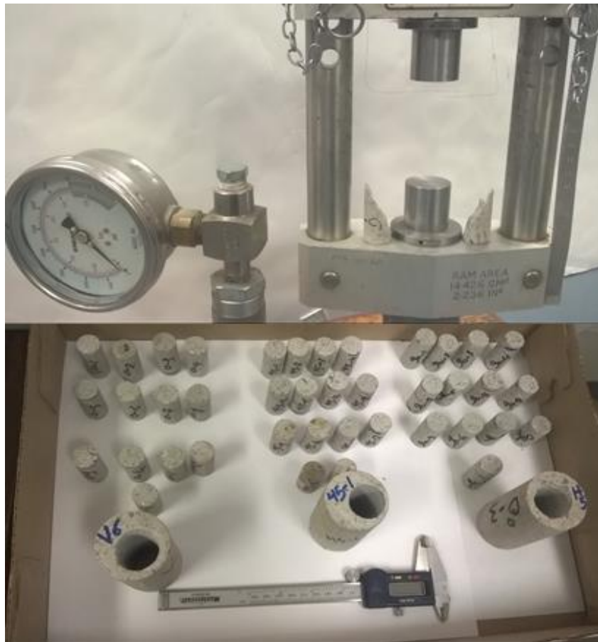
Figure 4-2. Calibrated point load index apparatus with flattened-steel-platens for OUCS test (top). OUCS RLM samples and the larger samples, from which the smaller samples were cored (bottom)
