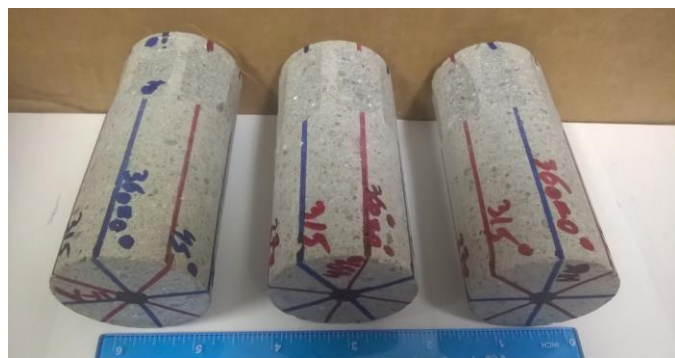
FIGURE 4. THREE RLM SAMPLES CORED IN THREE DIFFERENT ORIENTATIONS. EACH SAMPLE HAS PREPARED POSITIONS AT THE TOP ENDS FOR FULL CIRCULAR VP AND VS MEASUREMENTS
