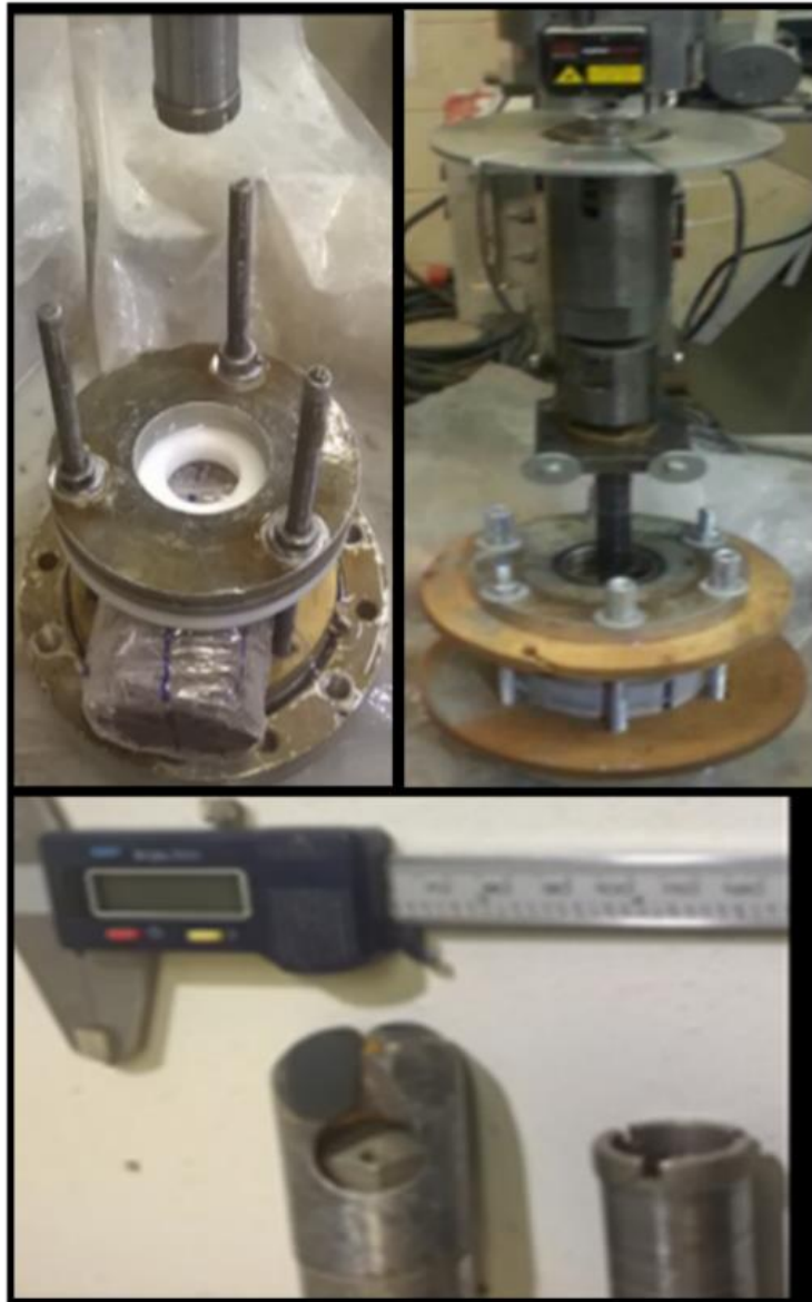
Figure 8-1. Apparatus for shale coring and drilling experiments with coring and drill bits
