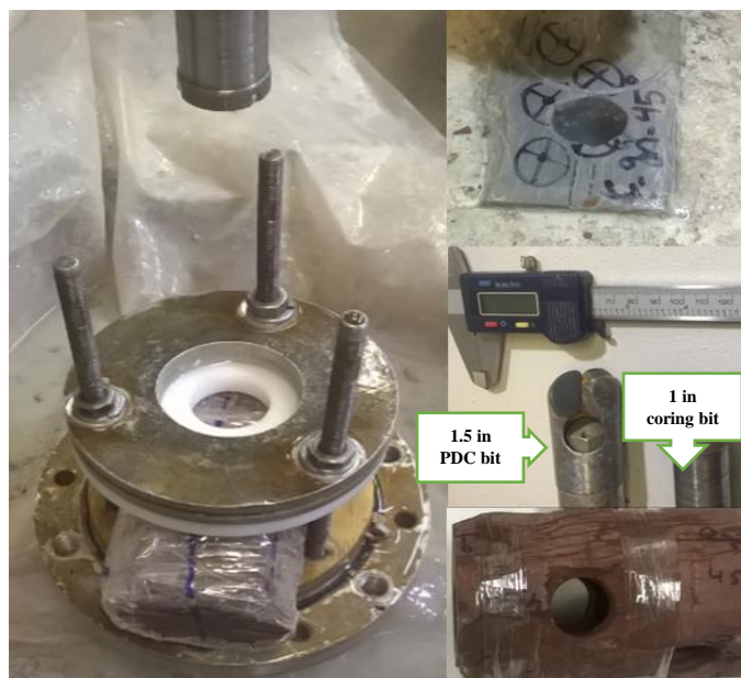
FIGURE 2. GREEN SHALE SAMPLE CAST AND DRILLED PARALLEL TO BEDDING USING 35 MM PDC BIT (TOP RIGHT). RED SHALE SAMPLE READY TO BE DRILLED (BOTTOM LEFT) AND RED SHALE SAMPLE DRILLED IN DIFFERENT ORIENTATIONS USING 25.4 MM DIAMOND CORING BIT (BOTTOM RIGHT)
