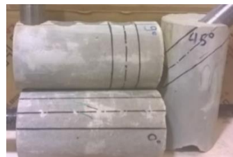
Figure 1. Three 152.4 mm diameter and 304.8 mm long, out of which 47.6 mm diameter RLM samples were cored
