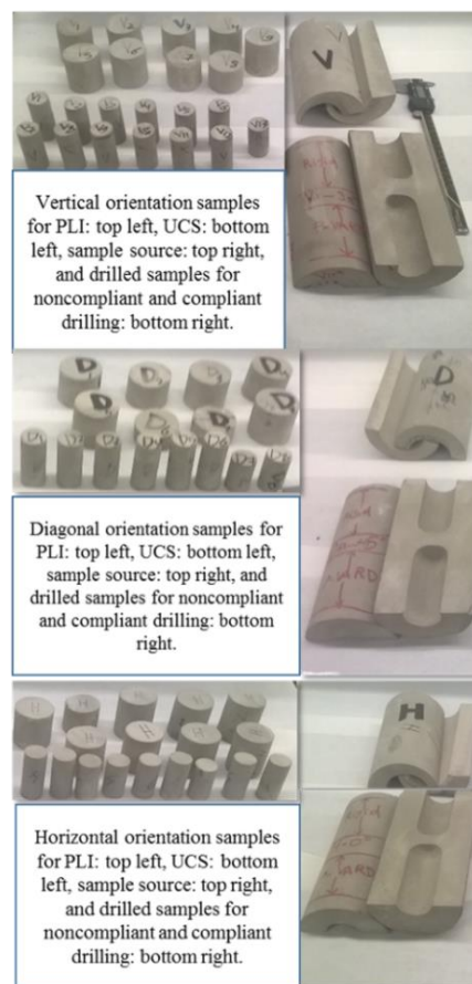
Figure 6. Samples for PLI and UCS before testing as well as drilled samples.
