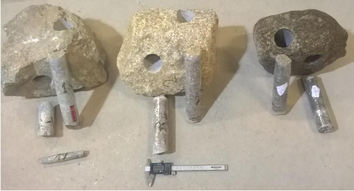
Figure 4-6. Granite rocks of different types with the obtained samples cored vertically and horizontally
