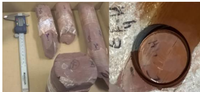
FIGURE 1. RED SHALE CORES IN DIFFERENT DIAMETERS. ALL SAMPLES ARE CORED PARALLEL TO THE SHALE BEDDING.
