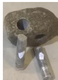
Figure 2. Granite (natural rock) after coring 47.6 mm diameter vertical and horizontal samples
