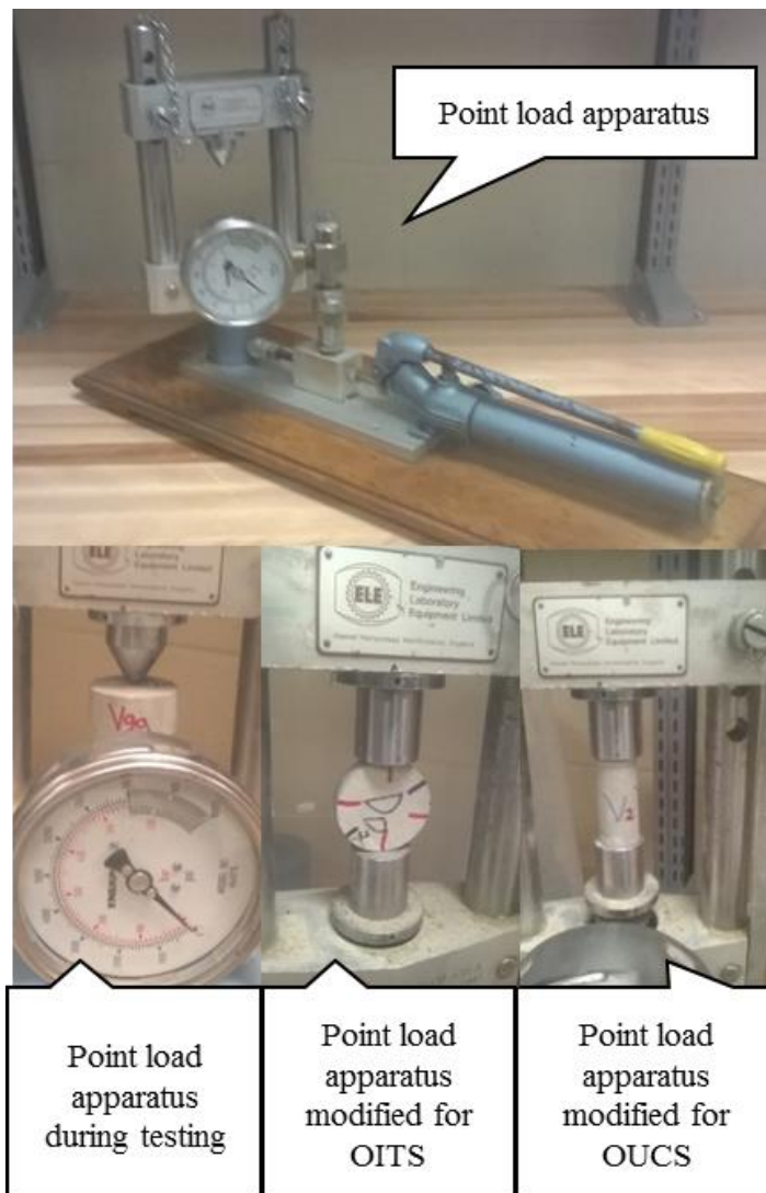
Figure 9-5. PLI Apparatus with modifications with flat-end pistons for OITS and OUCS
