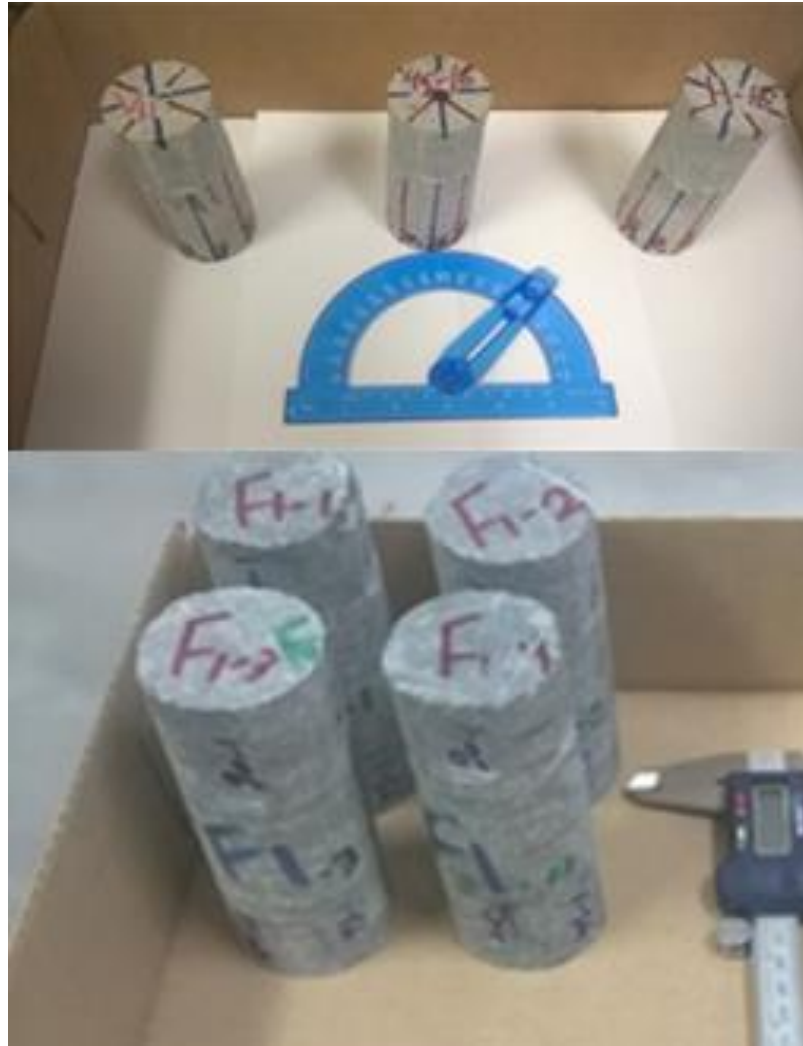
Figure 4-1. Three RLM samples were cored in three different orientations (top), four granite rock core samples cored in vertical and horizontal directions from granite rocks (bottom). All seven samples were cored using 50.8 mm diamond coring bit and have prepared positions (flat surface by a grinder) for full circular V_p and V_s measurements
