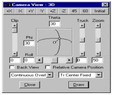
This interface involves two angles of rotation (theta corresponding to tilt, and phi corresponding to pan), zooming and tracking parameters, as well as a part of plot to be cipped. All these parameters can be controlled manually, by using mouse, and create an interactive viewing.
