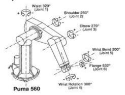
can be described by a matrix:  $X = P T_6 E$  where  $T_6 = A_0 A_1 A_2 A_3 A_4 A_5 A_6$ , and matrices  $A_i$  are varying only with joint angles, E is so-called tool transformation matrix, and P is a matrix which relates the coordinates and orientation of the robot arm base to the world coordinates.
