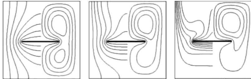
Fig. 3. Isotherms and streamlines for A = 0.5 , A_1 = 0.5 , Gr = 10^3, 10^4 and 10^5 .
