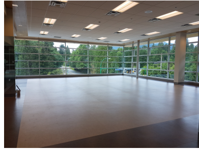
Figure 1.5: Examples of some challenging indoor environments in which visual localization methods are prone to failure. The environment in the left picture has repetitive features. In contrast, in the right picture, the room has a deficient number of features, which is inadequate for the robots to localize themselves successfully.
