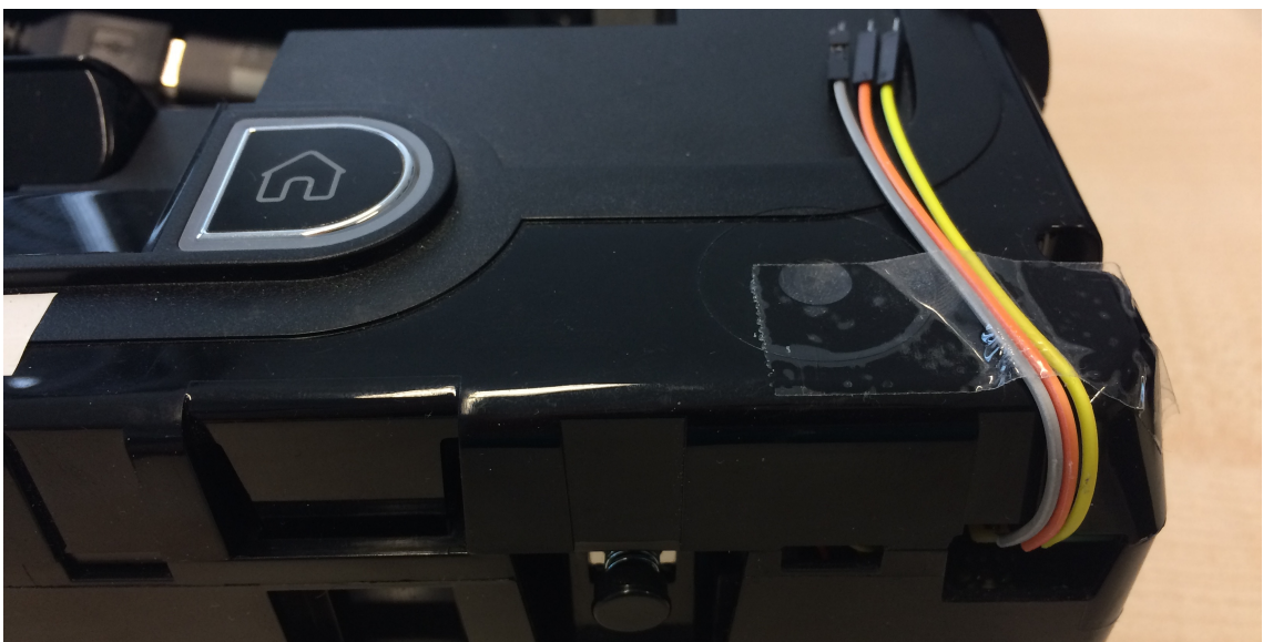
Figure 11: Unlabeled serial interface.
