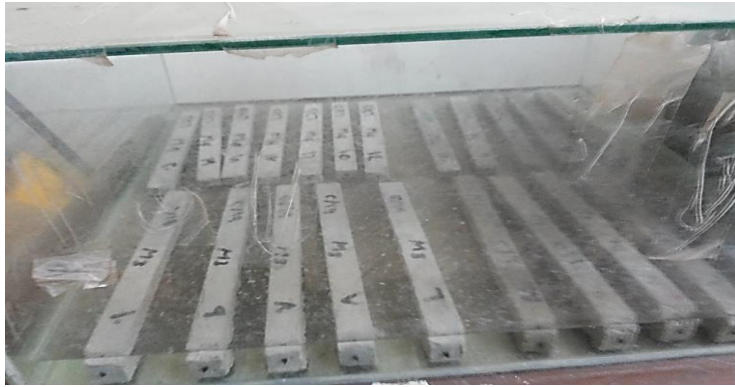
Fig. 10. Setup for sulfate attack test
