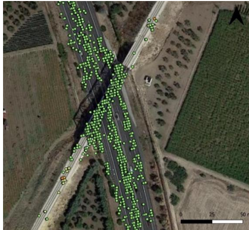
313 Fig. 7 – PS-outcomes from the InSAR analysis carried out on the truss bridge area
