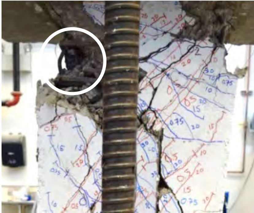
Figure B.28 – CB2AD with longitudinal bar buckling during second cycle to +5% chord rotation
