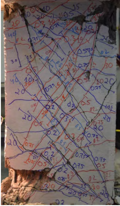
Figure B.15 – CB3D at target 4% chord rotation
