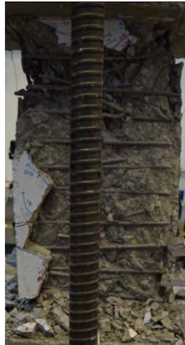
Figure B.18 – CB2D at target 5% chord rotation
