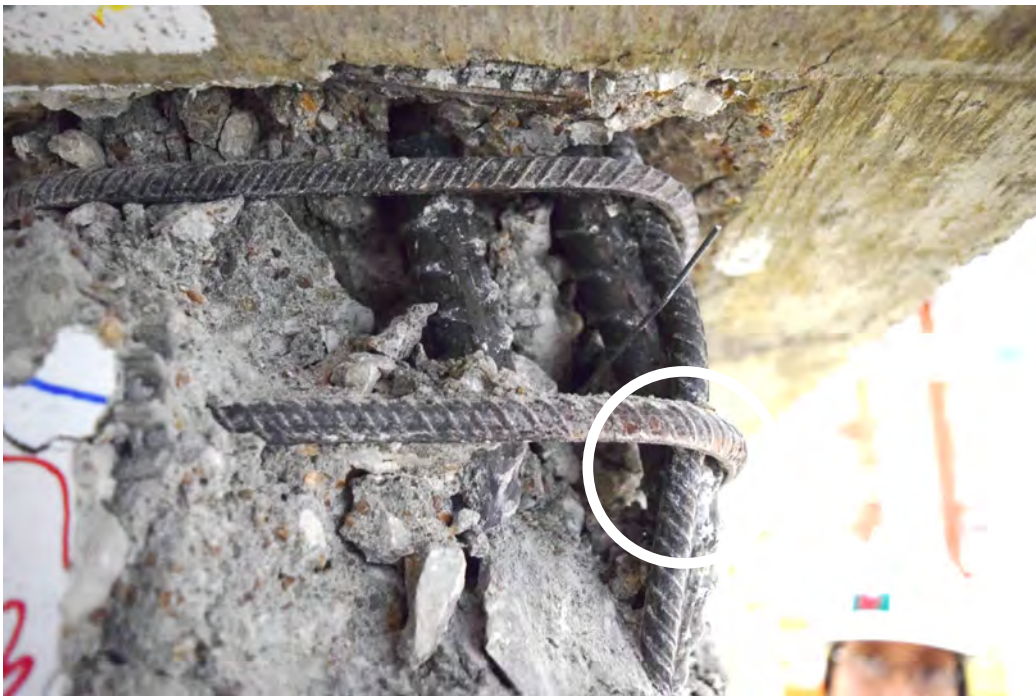
Figure B.24 – CB1 with longitudinal bar fracture during first cycle to +8% chord rotation
