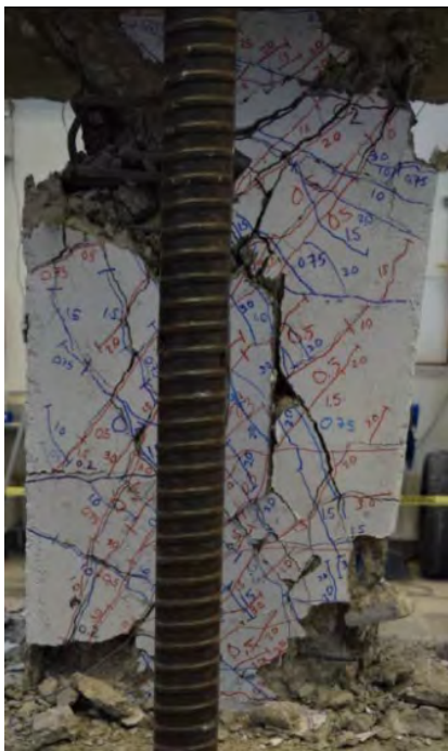
Figure B.18 – CB2D at target 5% chord rotation
