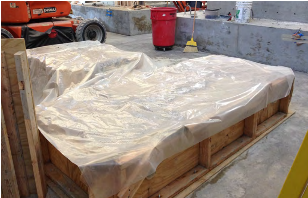
Figure A.10 – Curing of a coupling beam specimen
