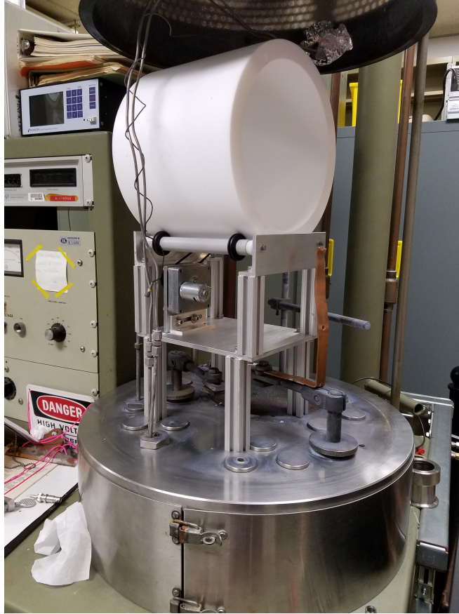
Figure 3.11: The platform designed for the TPB coating of the Teflon cylinders shown inside the evaporator. The Teflon cylinder rotates on the rollers which are powered by a small motor. The crucible, not seen here but in Fig. 3.12, is placed inside the cylinder such that the crucible is located the same distance away from the cylinder coating surface as in the previous test runs.
