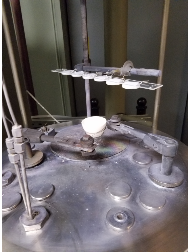
Figure 3.9: Operation of the bell jar evaporator at ORNL with test Teflon pieces to ensure that the TPB adhered to the Teflon surface before use on the Teflon cylinders in CENNS-10. The TPB is in the crucible (the ceramic bowl in the center) which is wrapped with tungsten wire and heated to a point where the TPB evaporates from the crucible.
