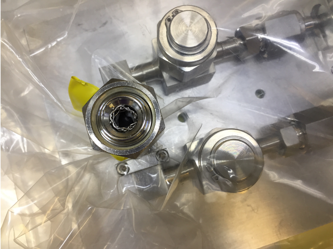
Figure 4.13: Activated carbon inside the source vessel after bake-out in a vacuum oven and before the ^{83}\text{Rb} deposition.
