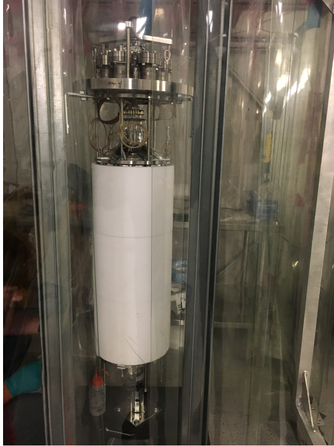
Figure 3.13: The CENNS-10 inner detector volume as constructed in Neutrino Alley after the upgrades described in this section. The three TPB-coated Teflon cylinder sections and the two PMTs make up the total active volume of the detector.
