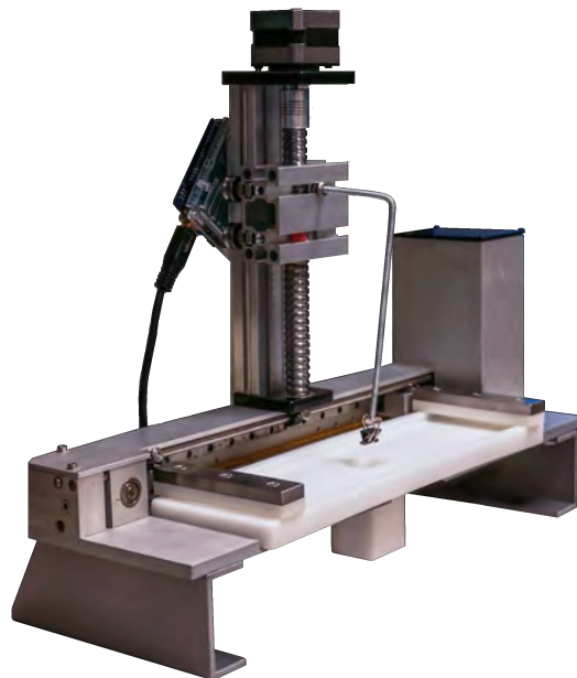
Figure 2.6. Automated Langmuir Blodgett Trough Deposition System. Although the metal base and barrier arms are original to the KSV Mini-trough system, the white dipping trough, dipping assembly with arm and sample holder, and microcontroller mounted on the back of the dipping assembly are specific to this project. Image by Sarah Dale.
