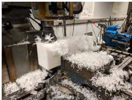
(a) Bulk material was removed from the work piece using the shell cutter tool. A large quantity of acetal chips are visible on the work piece mounting block.
