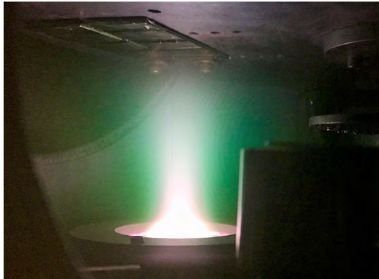
(b) Magnetron sputtering Cu onto glass substrate covered in Al foil masks. The discharge plasma is clearly visible, and has a bright green glow along the outer edges, and a violet glow beneath the cathode ring (barely visible in this image at the base of the plasma beam).
