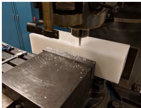
(b) The top of the trough containing the film area was created using pocket milling with an end mill tool.
