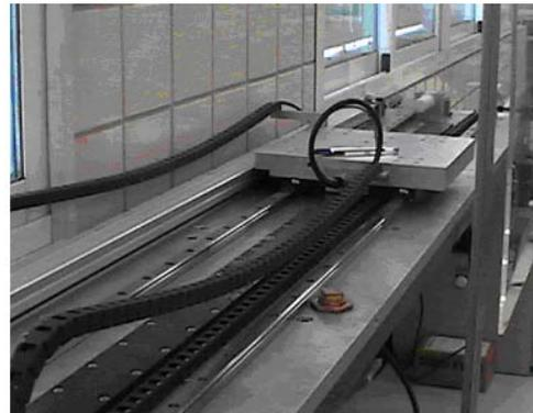
Figura 1: Motor lineal 1FN 3 de Siemens.
