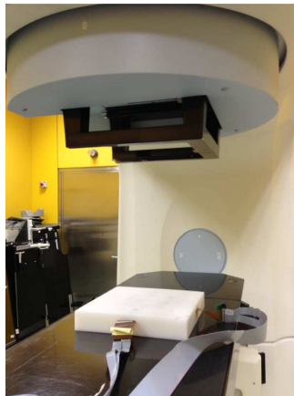
Figure 3: Dual SSSSD chip placed into a slab phantom and positioned on the treatment couch to be irradiated by the linac at the Hospital.
