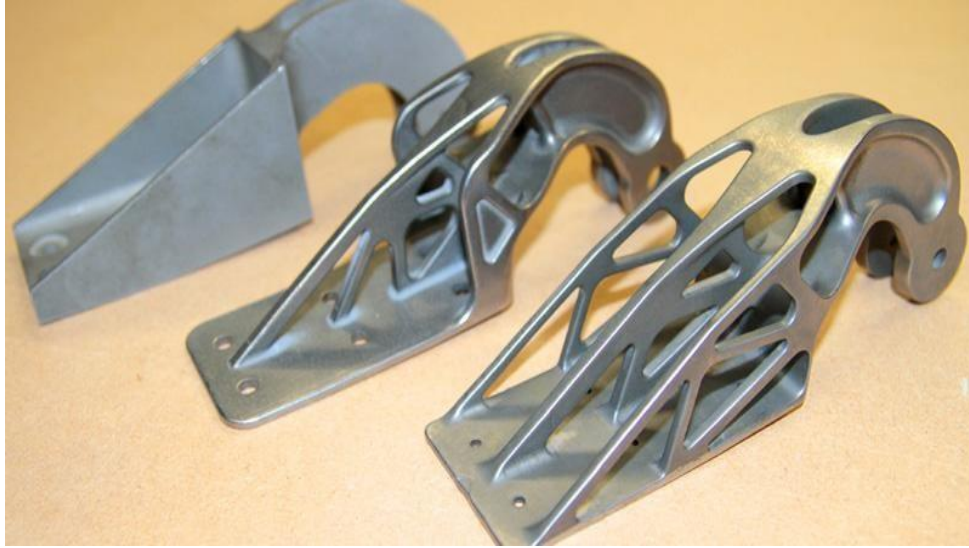
Figure 2-5 : A image taken at European Space Agency Conference which was used to describe the minimizing of weight of a product by redesigning the product geometry [49]
