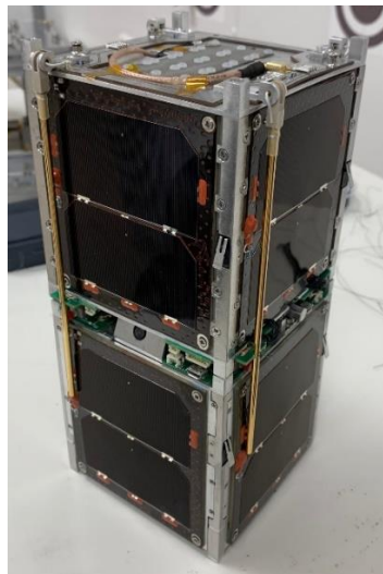
Figure 7. 11: Final assembly of 2U DESCENT satellite
