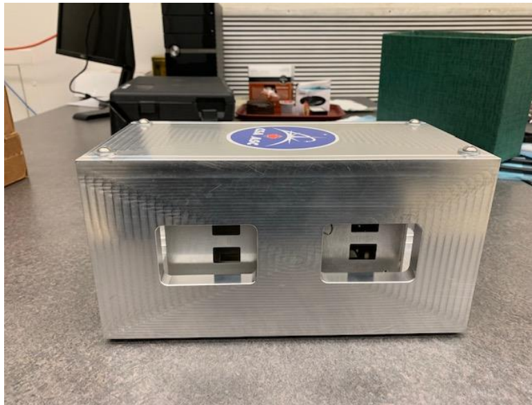
Figure 7. 9: Fit check of combined 2U DESCENT spacecraft
