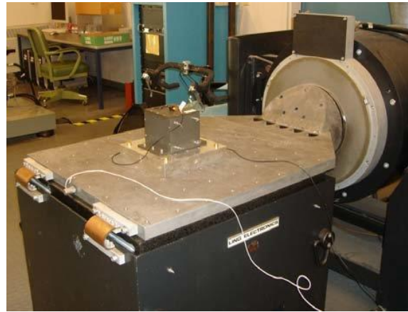
Figure 8. 3: Vibration table used for CubeSat Testing [32]
