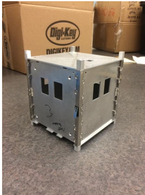
Figure 7. 3: Dry assembly of daughter spacecraft structure
