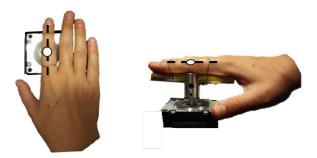
Figure 2.2: Two photos of the author's hand attached to the motor. During the experiment the motor rotated the participant's finger about the proximal interphalangeal joint (denoted by a white oval).
