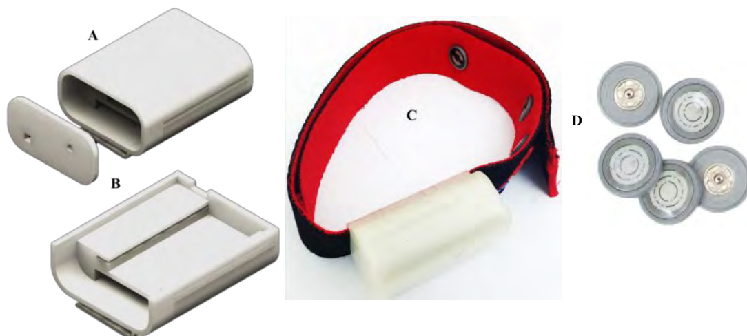
Figure 3. Exterior (A) and interior view (B) of the three-dimensional (3D) model of the electrocardiograms (ECG) amplifier and (C) the ECG amplifier with the chest belt and (D) dry electrodes.
