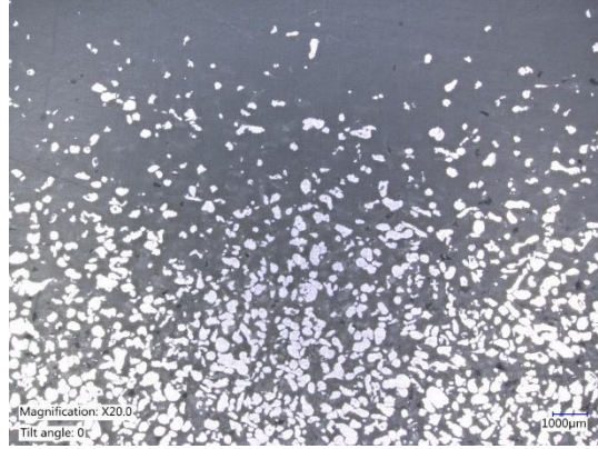
Figure 32 Microstructure of the FGM panel containing aluminum particles dispersed in the HDPE matrix with the concentration changing in the thickness direction
