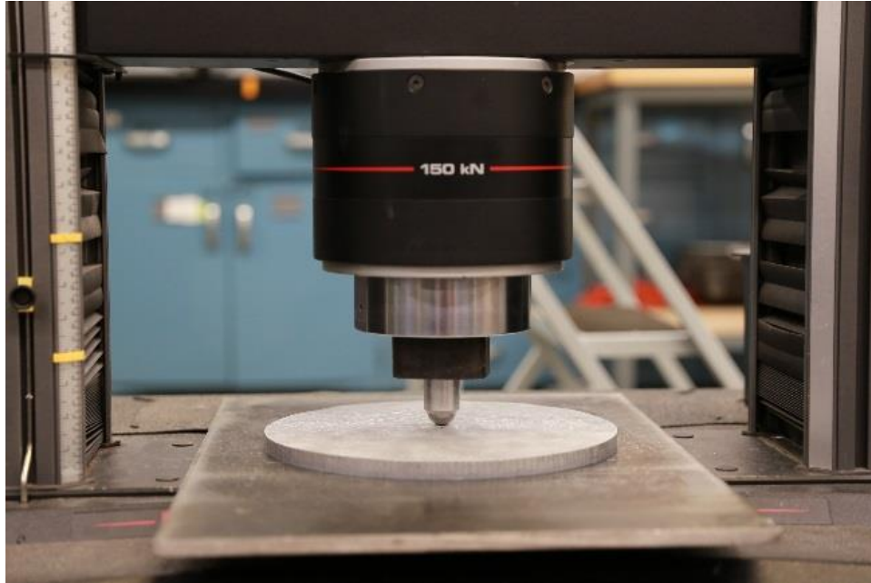
Figure 38 Point-load compression test on the curved FGM panel.
