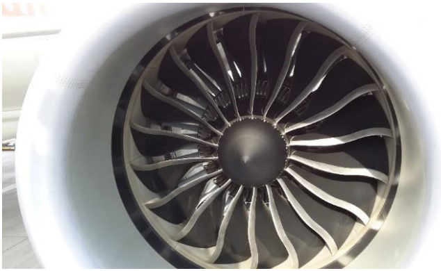
Figure 1.8: General Electric GE90 jet engine, with its 18 fan blades.
