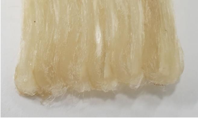
Figure 3.14: The combined effect of partially overlapping composite tracks and tow pull-up in regions of high path curvature.
