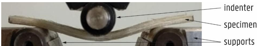
Figure 4.2: Setup of a flexural test, the specimen being under a flexural load.
