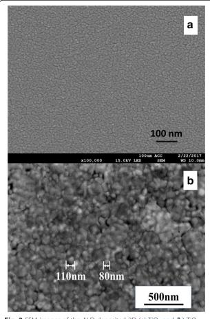
**Fig. 3** SEM images of the ALD-deposited 2D (a)  $TiO_2$  and (b)  $TiO_2$ - $Ga_2O_3$  heterostructure nano-films
