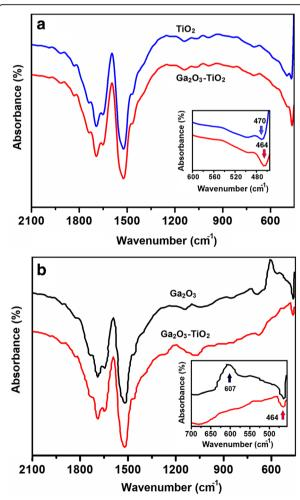
**Fig. 6** FTIR spectra of ALD-fabricated 2D  $\text{TiO}_2$  and  $\text{TiO}_2\text{-Ga}_2\text{O}_3$  n-p heterostructures (**a**) and 2D  $\text{Ga}_2\text{O}_3$  and  $\text{TiO}_2\text{-Ga}_2\text{O}_3$  n-p heterostructures (**b**)
