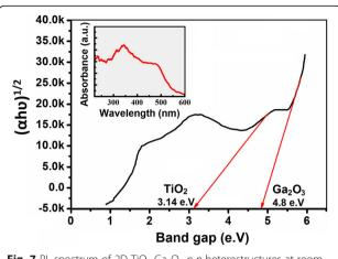
**Fig. 7** PL spectrum of 2D  $TiO_2$ - $Ga_2O_3$  n-p heterostructures at room temperature with bandgaps for  $TiO_2$  and  $Ga_2O_3$
