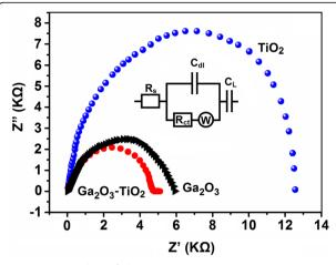
**Fig. 5** Nyquist plots of the 2D TiO $_2$ , Ga $_2$ O $_3$ , and TiO $_2$ -Ga $_2$ O $_3$  heterostructures tested in air at a temperature of 25  $^{\circ}$ C
