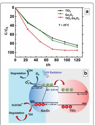
**Fig. 8** MO degradation efficiency for 2D TiO<sub>2</sub>,  $Ga_2O_3$ , and  $TiO_2$ - $Ga_2O_3$  n-p heterostructures under  $\lambda = 254$  nm UV light (**a**). Schematic photocatalytic reaction process and charge separation transfer of 2D  $TiO_2$ - $Ga_2O_3$  under UV light irradiation (**b**)
