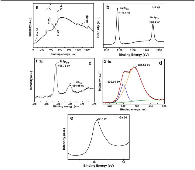
**Fig. 4** XPS spectra of 2D TiO<sub>2</sub>-Ga<sub>2</sub>O<sub>3</sub> *n-p* heterostructures. **a** Full survey scan spectrum. **b** Ga 2p region. **c** Ti 2p region. **d** O 1s region. and **e** Ga 3d region
