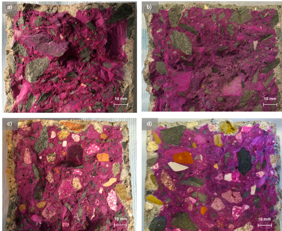
Fig. 6. 56 d carbonation front in specimens exposed to CO 2 at a concentration of 1%: a) RRC; b) NC; c) RRC-50; d) NC-50.
