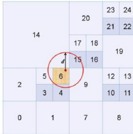
Figure 2 [29] – Finding neighbors for a given point using a Quadtree
