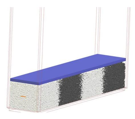
Figure 5.5: Numerical pullout test visualization for  $C_u = 3$
