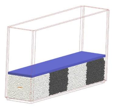
Figure 5.1: Numerical pullout test visualization for  $C_u = 1$
