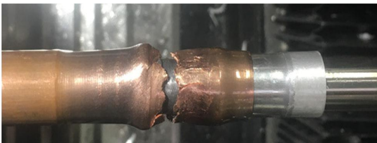
Fig. 14 Fracture of bimetal tube
