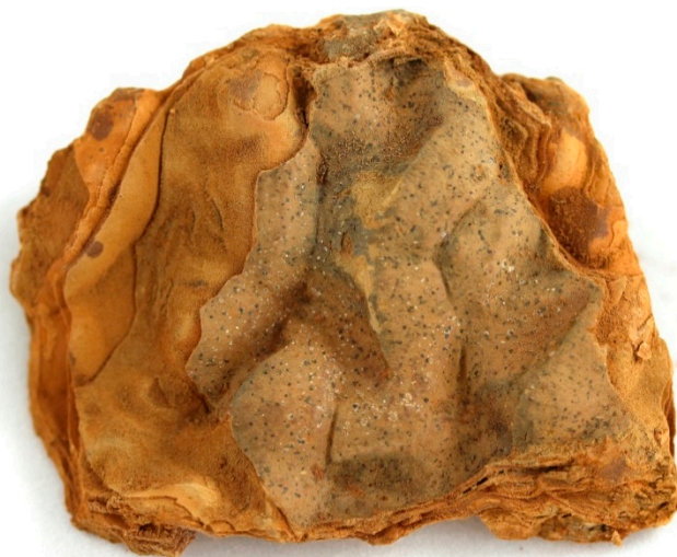
Figure 2. Example of beige incrustation from a drainage pipe with Ra-rich baryte. Size 6 \times 5 \text{ cm}^2 .
