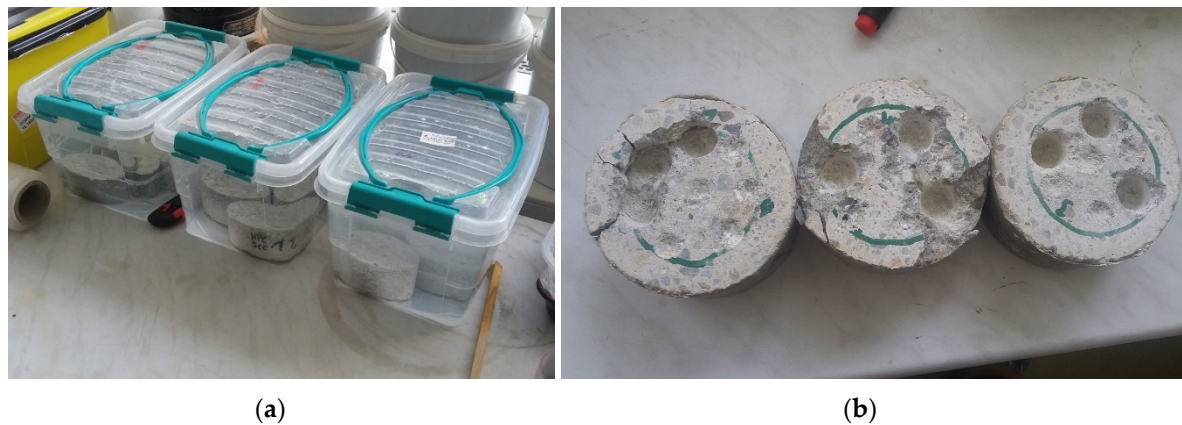
Figure 5. The process of the modified NORDTEST NT Build 443: (a) samples submerged in the chloride solution; (b) samples after drilling.
