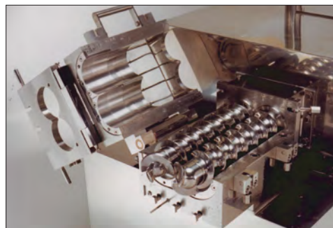
The patented hemispherical shaped dies result in evenly distributed extrusion forces.
