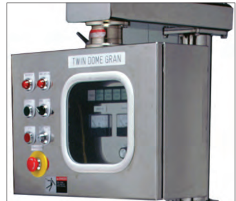
Integrated controls are mounted on an articulating arm.
