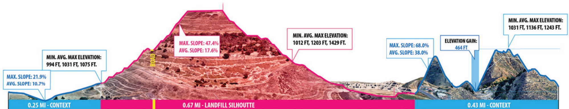
[186] W-E Longitudinal Profile of Calabasas Landfill.
