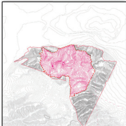
[248] Contour map and cutout surface with of modified landfill surface P1 (Zhong 2020).
