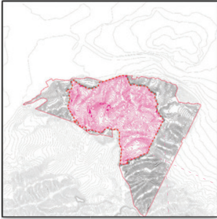
[251] Contour map and cutout surface with of modified landfill surface P4 (Zhong 2020).
