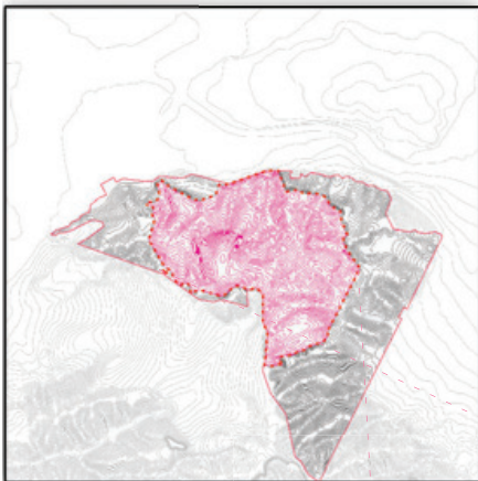
[252] Contour map and cutout surface with of modified landfill surface P5 (Zhong 2020).
