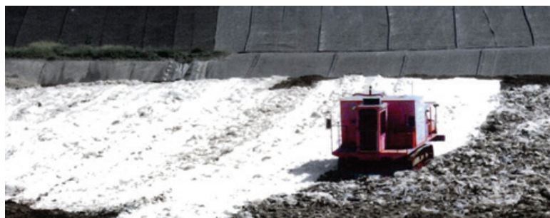
[23] Existing Daily Cover Operations Using Foam in Puente Hills Landfill (LACSD 2001).
