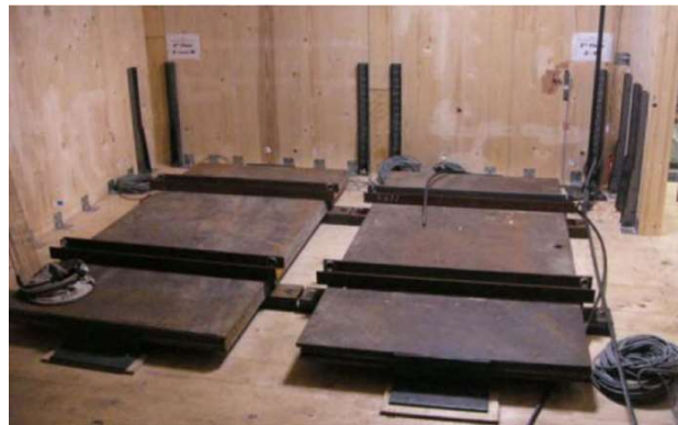
B) Additional steel plates for added load
