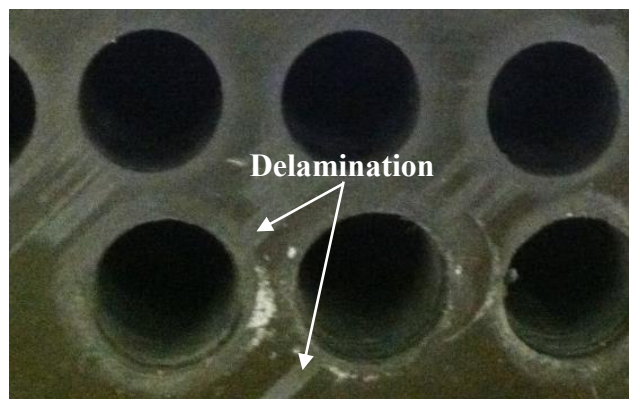
Figure 2.26 Delamination in exit surface of CFRP
