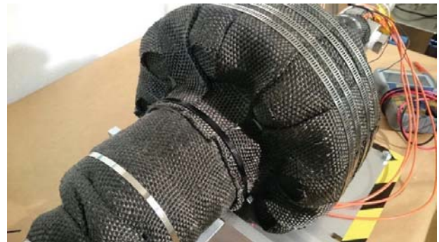
Fig. 9 Thermal insulation material cover
