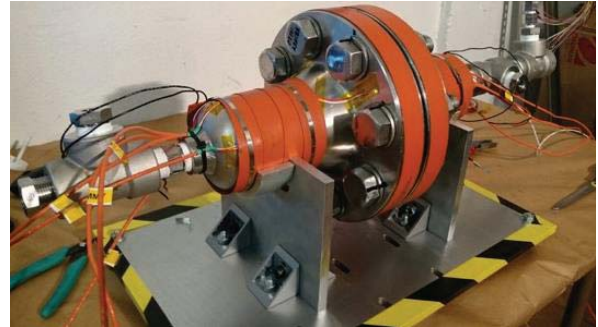
Fig. 8 View of the ‘Supercritical Chamber’. The orange tapes that surround the structure correspond to the heating strips through which the thermal cycle is applied. The external Pt100 temperature and strain gauge sensors attached to the chamber skin are visible, with the PID control at the clamp
