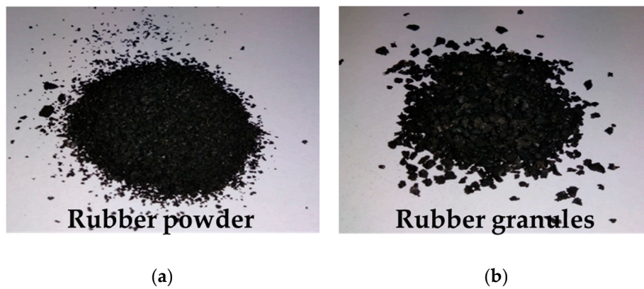
Figure 7. Size and shape of GTR powder (a) and granules (b) used in the research work.
