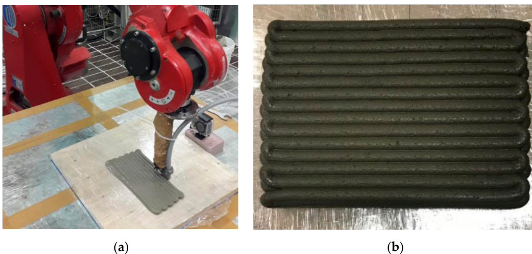
Figure 8. Printability test: slab extrusion process (a) and consistency of the optimum fresh mix (b).
