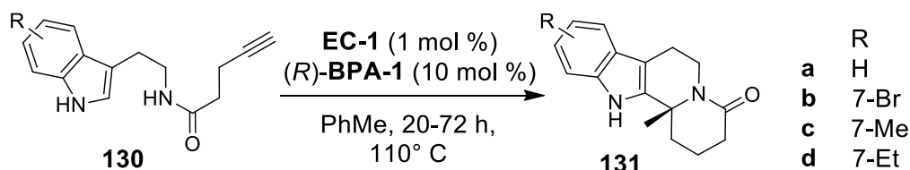
Scheme 38. Synthesis of \delta -lactams via 6- exo -cyclization cascade.
