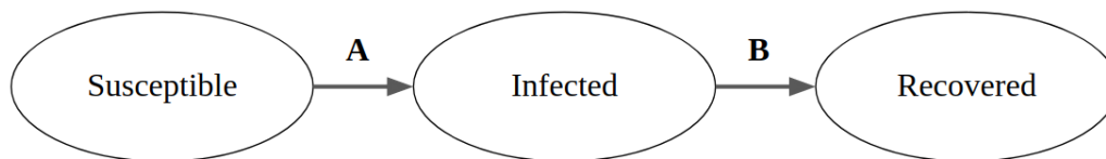
Figure 1. States and transitions of the Susceptible-Infected-Recovered (SIR) model. The same are used in EPIC, and they refer to a specific message. Let us identify it as M , which is sent in the VANET. Each vehicle that never received the message M is in the susceptible state. When it receives the message M , it makes a transition to the infected state, setting a timer \Delta t . Once the timer expires, the vehicle decides whether to rebroadcast a message or not (this is part of the EPIC algorithm and is described in the following) and makes a transition to the recovered state. When a vehicle is in this latter state, it discards all the next copies of M .
