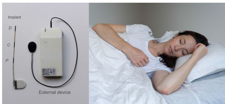
Fig. 5 Illustration of the subcutaneous recordings system. Left: illustration of the implant and the beta-version of the external device used to collect data in the present study. The placement of the Proximal ( P ), Center ( C ) and Distal ( D ) electrodes are indicated by the letters. The length of the implant is approximately 11 cm. Right: illustration of the commercially available device. The device is worn under the shirt and secured in place by a magnet (gray circle)
