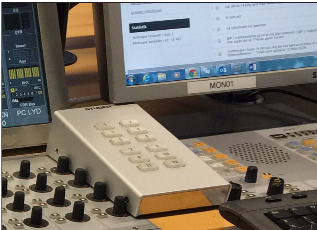
Picture 34: Twelve buttons are connected to the numbered buttons on the sound screen (in box no. 8)
