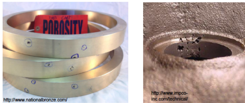
Figure 1.3: This figure shows porosity defect in a cast bronze bar stock [3].
