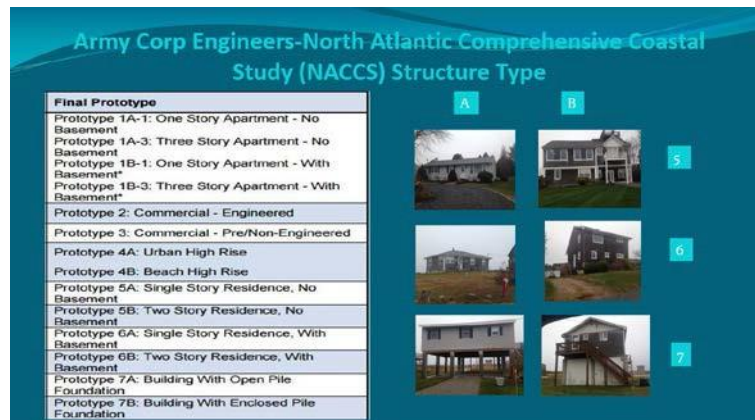
Figure 4. Army Corp of Engineers (ACOE) North Atlantic Coast Comprehensive Study (NACCS) structure types (left side). Photographs of structure prototypes 5, 6, and 7, categories A and B are also shown (right side). 5 and 6 are residences, without and with basements; while A and B refer to single and two story buildings, respectively. Prototype 7 have pile foundations, A—open piles and B—enclosed pile. Reproduced from [1], with permission from MDPI, 2020.
