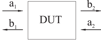
Figure 2.4: The incident and reflected waves passing through the Device Under Test (DUT).
