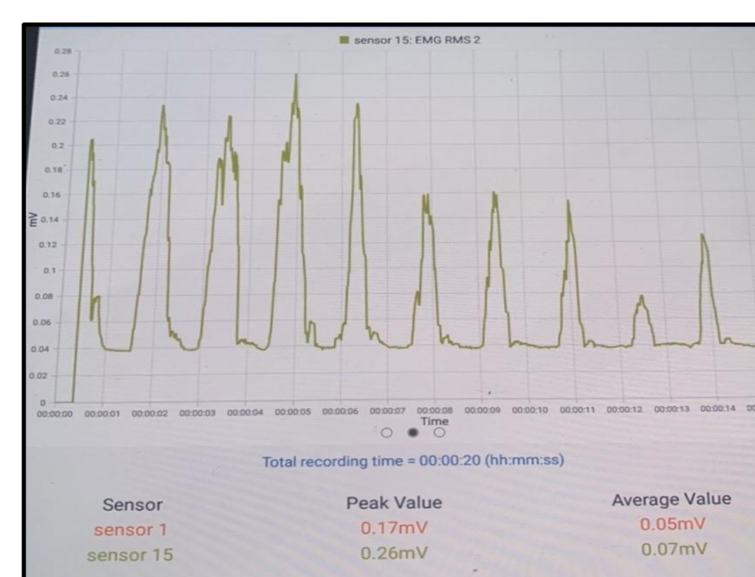
Figure 3. Graph of voltage from action potentials measured by EMG sensor with repeated muscle contractions
