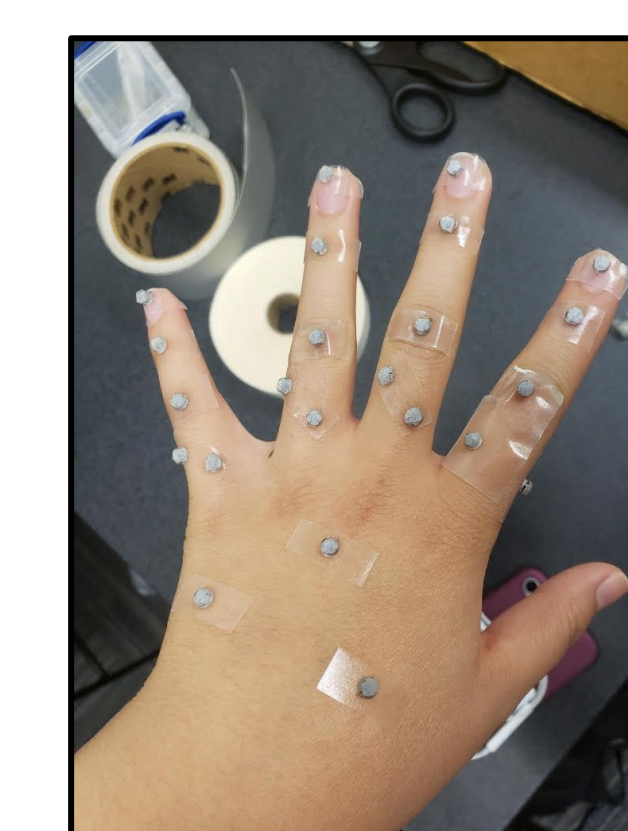
Figure 4. Reflective sensor placement on fretting hand
