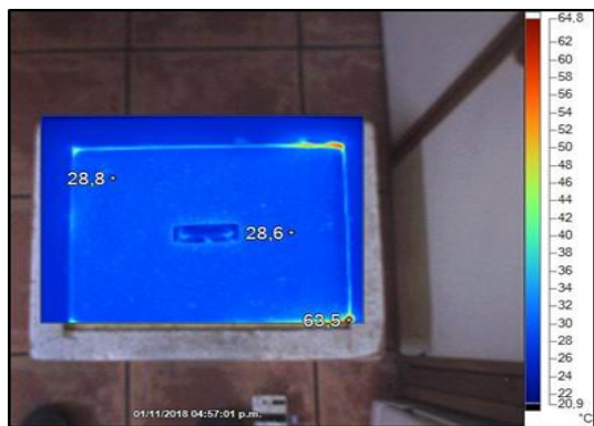
Figure 15. Top thermography of parallelepiped HRB
