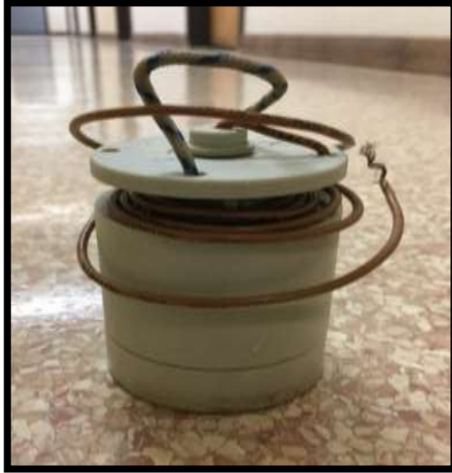
Figure 8. The saturated lead chloride non-polarizing electrode that we used.
