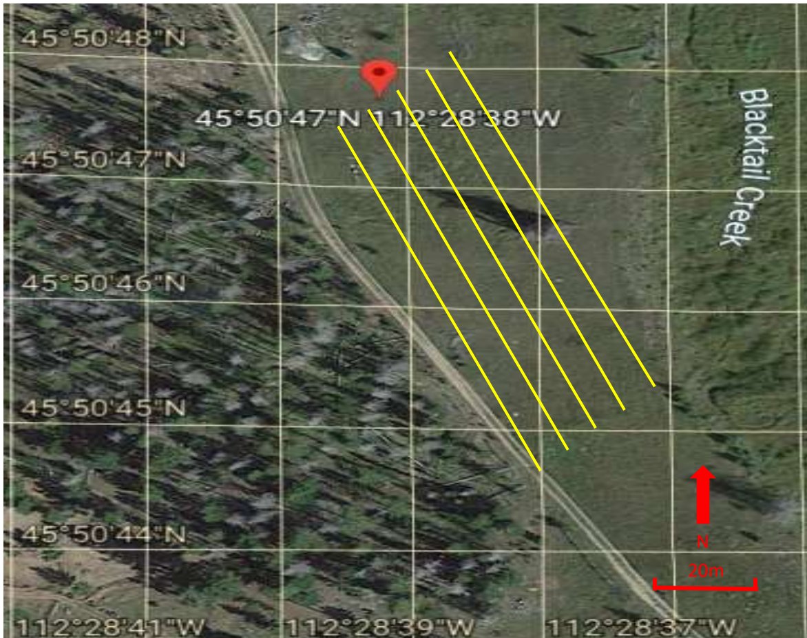
Figure 7. 3D resistivity and self-potential layout indicated by yellow lines
