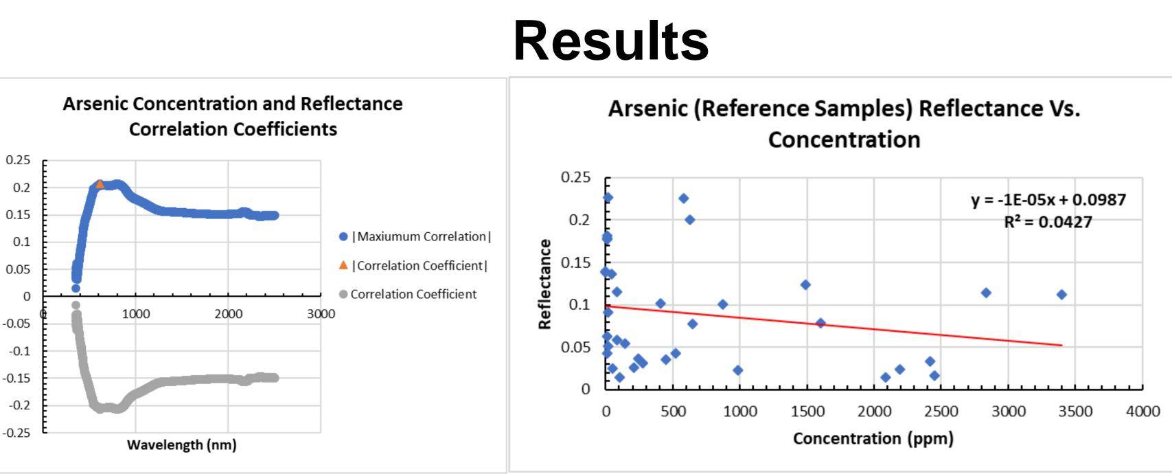
**Above (left)** is a plot of correlation coefficient vs. wavelength. The correlation coefficients were calculated in MATLAB and plotted in Excel. Above (right) is a plot of reflectance vs. concentration for the maximum correlation wavelength and the best fit linear relationship determined in Excel. Both of the above results are for the element arsenic from the reference samples with a known concentration.
