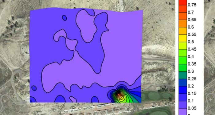
**Above (left)** is the concentration of zinc measured by LIBS in % and (right) calculated by the reflectance and information from the reference sample data in ppm.
