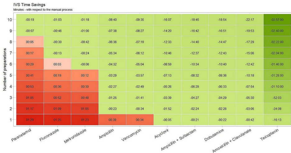
FIGURE 4 | Estimated time savings. I.V. Station ® expected time-saving compared to manual preparation. With a low number of doses, I.V. Station ® could result in more time-consuming than the manual method (red boxes). With the increase of preparations, I.V. Station ® leads to a progressive optimization of the preparation process (green boxes).
