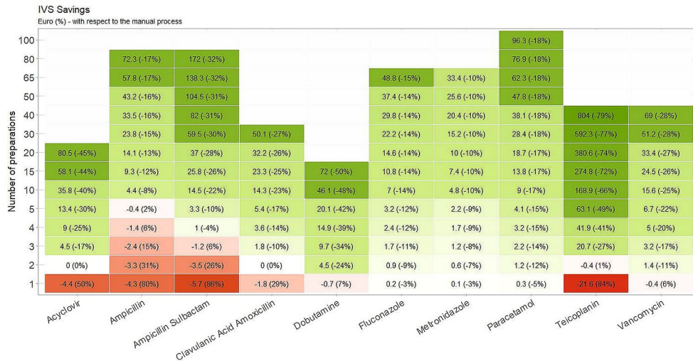
FIGURE 2 | Estimated cost savings. The robotic preparations result more expensive than the manual one in the red boxes. As the amount of preparations increases, I.V. Station® leads to an optimization of materials consumption and costs, becoming equal to manual preparation (white boxes) or even less expensive (green boxes).
