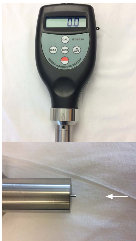
Fig. 4. Shore A durometer. The arrow indicates the device indenter.
