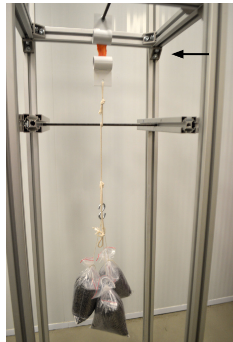
Fig. 1. Testing frame set-up. A standing frame with custom clamps secured superiorly and inferiorly with a suspended 3-kg weight and stabilizing bar. The arrow indicates the location of the glenohumeral joint capsular tissue prior to application of the gelatin pad.
