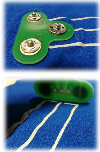
Figure 2. a) PCB with snap buttons soldered on top (top). b) Connection between PCB and fabric via 8331-B epoxy (bottom)
