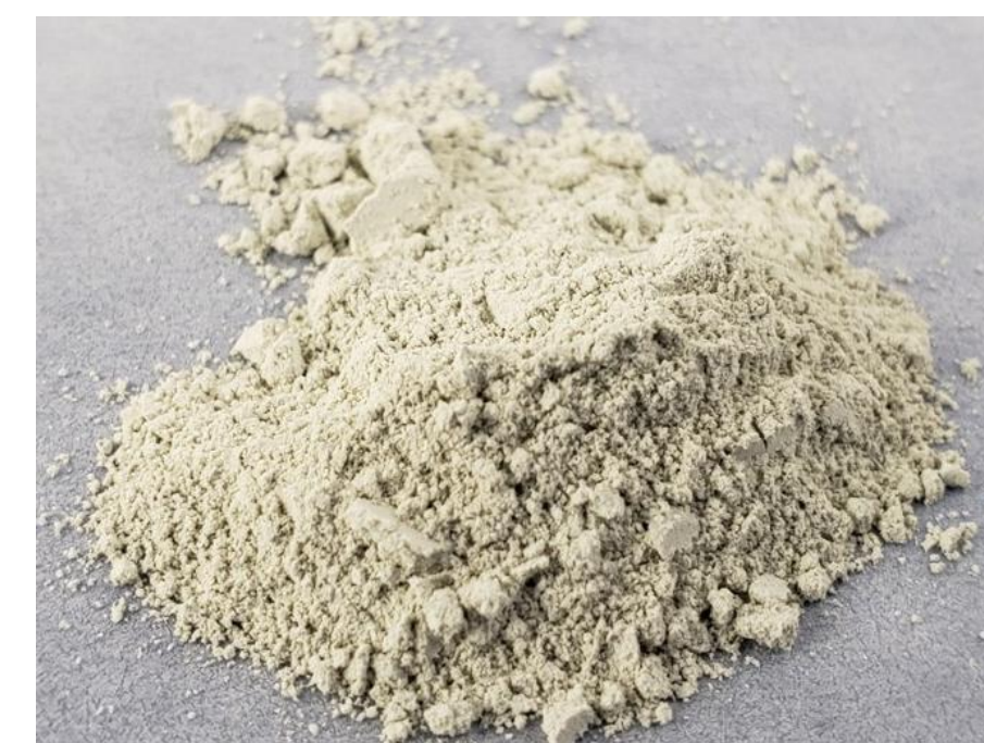
Fig.3. Milled 500 ppm MnO_2 -doped CeO_2 powder. Pure, 1000, and 2500 ppm samples were also fabricated.
