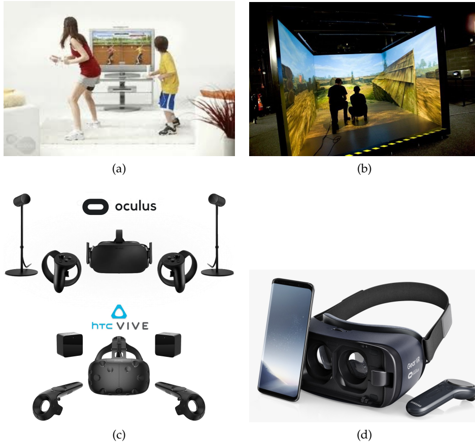
Figure 2: Examples of non-immersive (a) and immersive (b, c, d) VR systems. (a) Non-immersive setup based on Nintendo Wii. (b) A room filling technology, the CAVE. (c) Two head-mounted displays, the Oculus (top) and the HTC Vive (bottom). (d) The Gear VR, a mobile headset.
