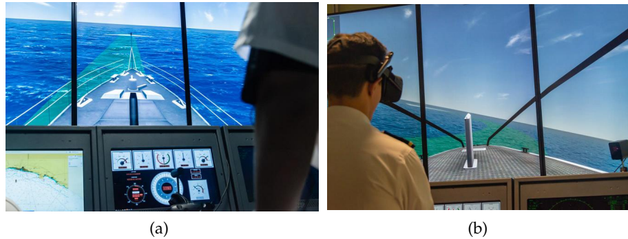
Figure 59: Industrial use case: the two visualization modalities of the ship handling simulator: (a) non immersive with monitors and (b) immersive with the HMD.
