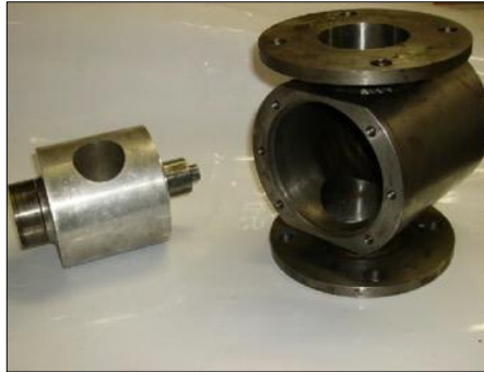
Fig. 2.7 – Rotating Valve Used in the Pulse Generator System
