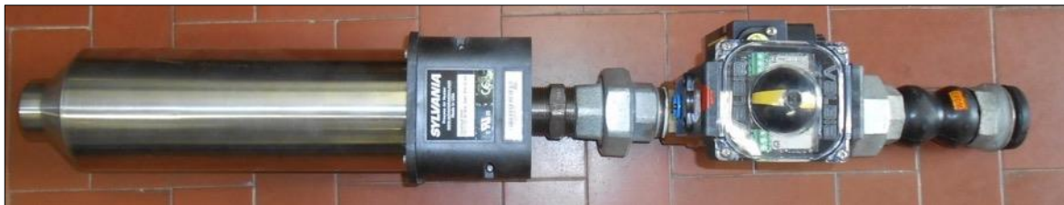
Fig. A.3 – A Single Electrical Heater Element and Electro-Pneumatic Valve
