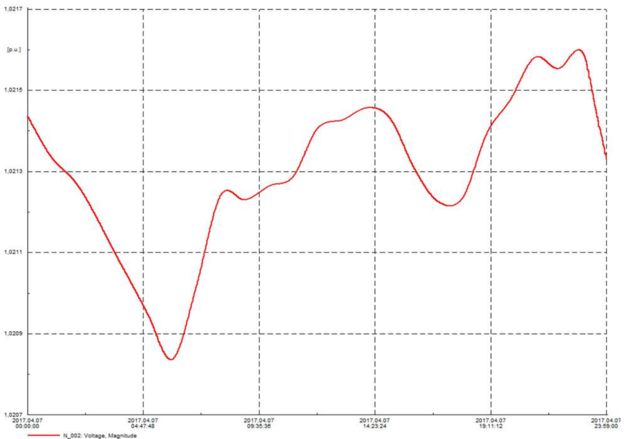
Figure 19: Node 2 Voltage in PU
